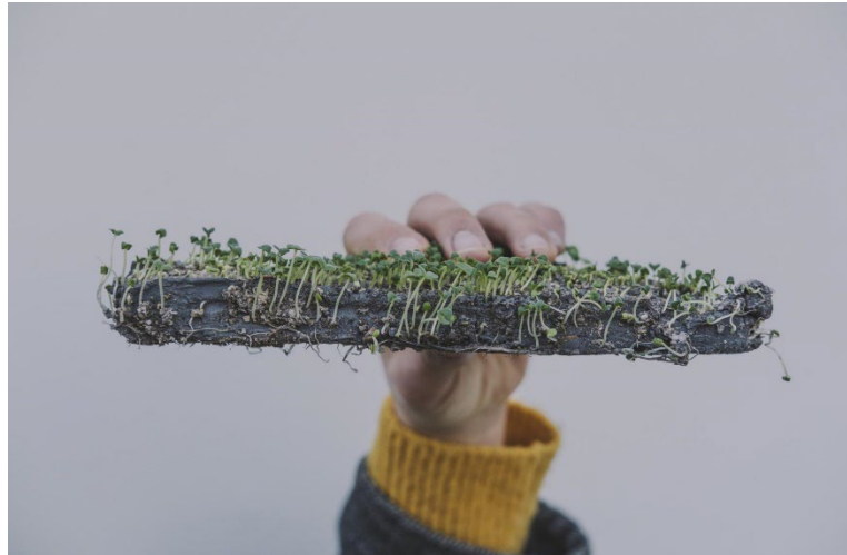
Figure 6 First experiments of vegetated tiles with quinoa seeds (Source: Authors)
